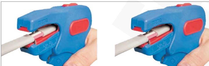
Stripping external insulation
