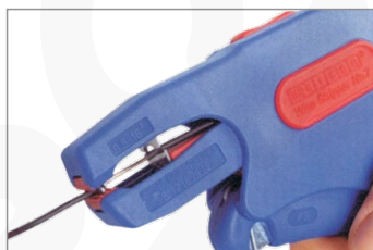
Stripping internal insulation
