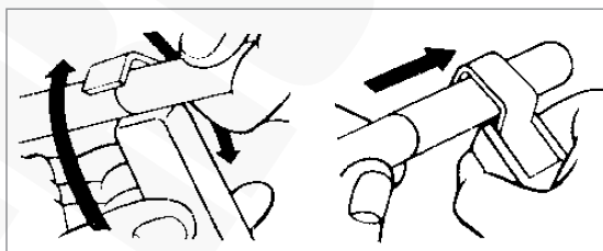
Stripping insulation from the end of cable
