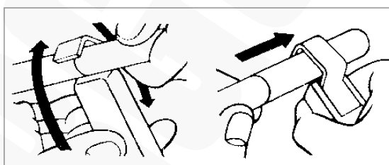
Stripping insulation from the end of cable
