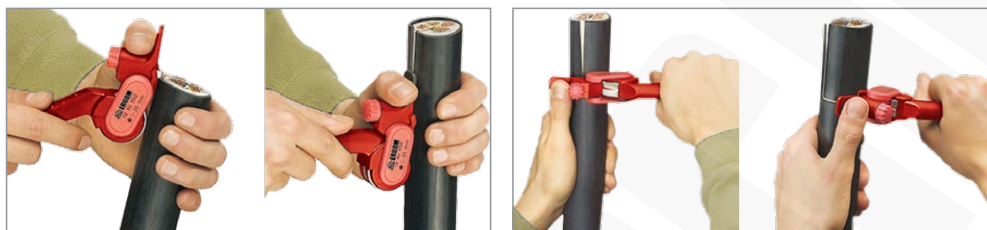
Longitudinal insulation cutting
