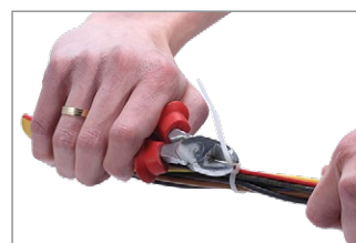
1.4 - Cut the exceeding part of the tie with the tool, leaving a few mm length as safety
