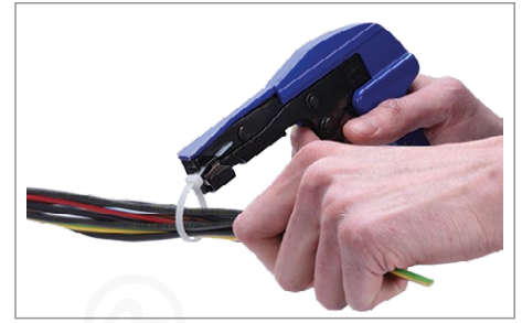
2.2 - Grip the cable tie with the tool
