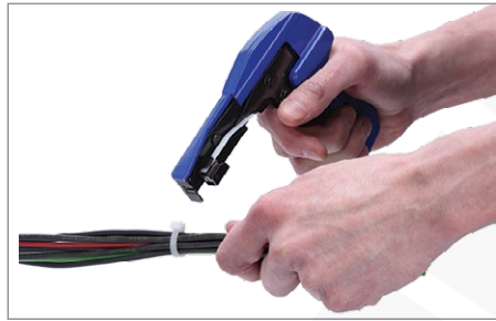
2.4 - Cut the exceeding part of the cable tie, properly adjusting the setting of the tool
