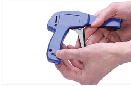
2.1 - Tightening the cable ties with a tool - set the max tension of the tool depending on the size of the tie
